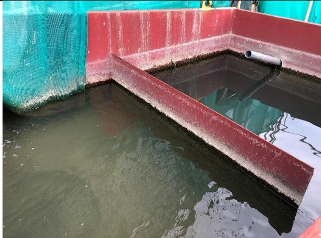
Sedimentation was enhanced for the silt removal.
