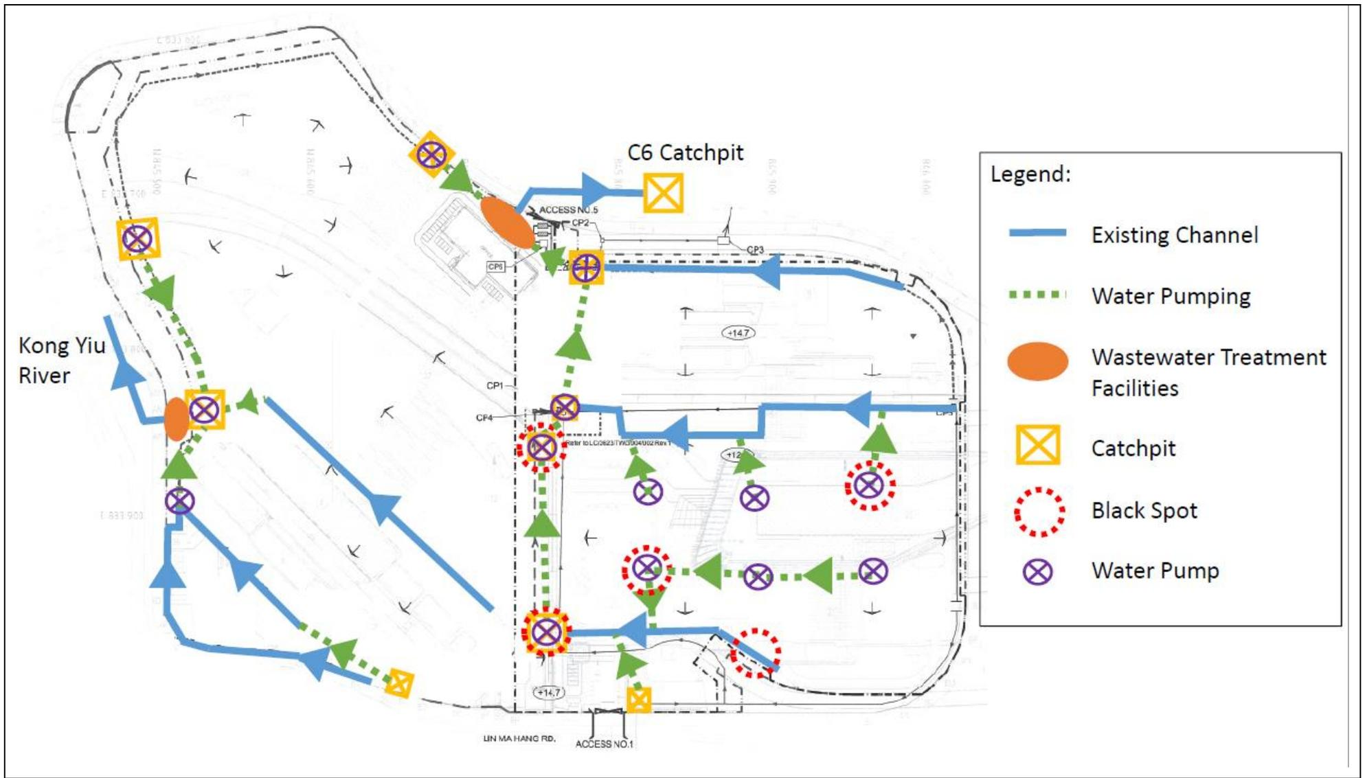
**Figure 3 Drainage Plan**
