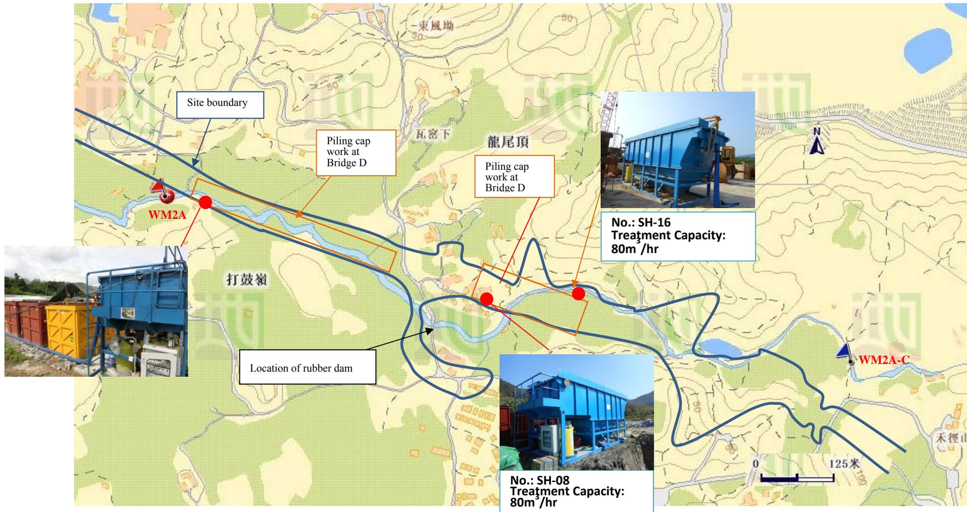
Figure 1 Location Map for Water Quality Monitoring Locations WM2A, WM2A-Control and work area under Contract 6
