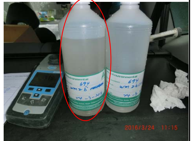
Photo 4 The water samples collected at WM2B on 24 March 2016 was slightly turbid.
