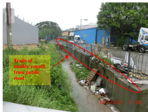
Photo 1 During water sampling on 21 March 2016, shallow water was observed at WM2B and the water quality at WM2B was turbid.
