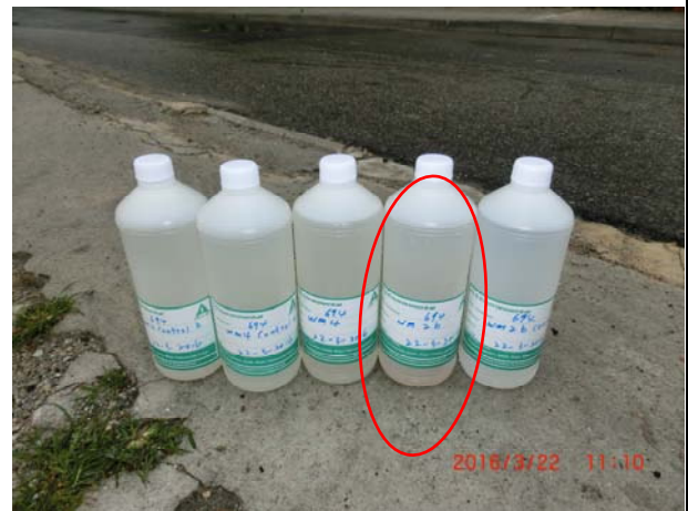
Photo 4 The water samples collected at WM2B on 21 March 2016 was slightly turbid.
