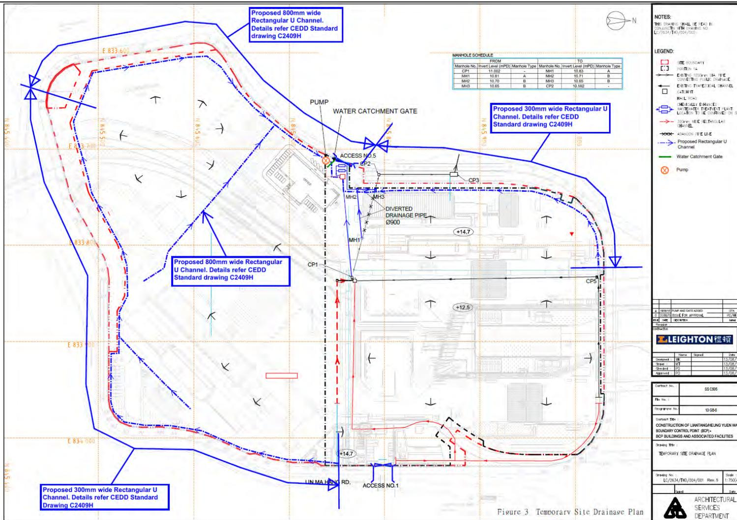
**Figure 3 Drainage Plan**
